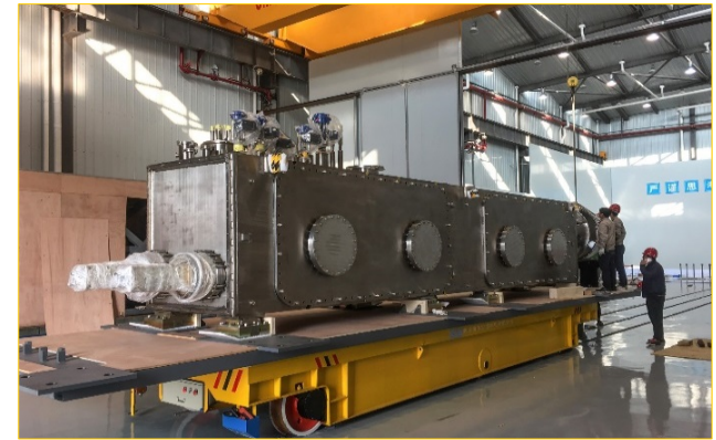
Magnetic Coil Feeders 1600 tons of equipment delivered
