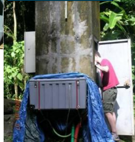
LISST installed on Capesterre River
